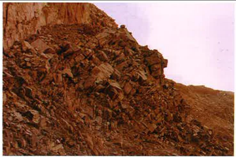
Figure 10.8: Bench scale block toppling on joints in granodiorite
