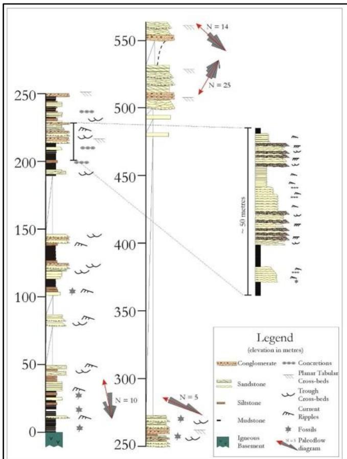
**Figure 15** Stratigraphic logs of the Eocene-Oligocene Huntingdon Formation.
