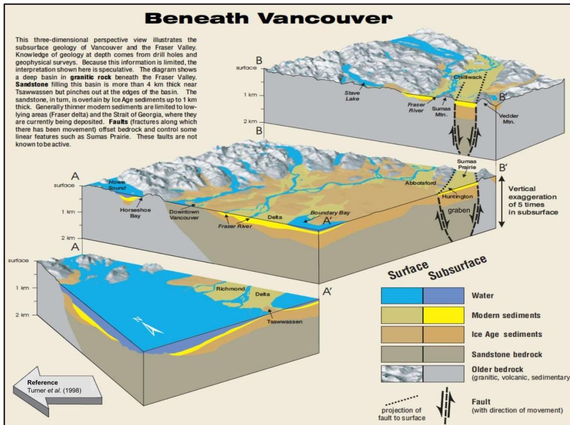
**Figure 8** Schematic 3D block diagrams showing the relationship of surface and subsurface bedrock, unconsolidated surficial sediments and water in the Sumas Mountain – Abbotsford area (modified from Turner et al. 1998).
