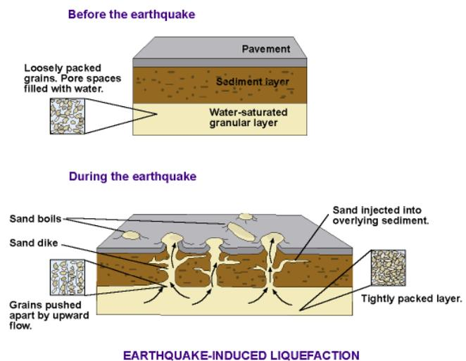
**Figure 9** Liquefaction process in water-saturated sediments.
