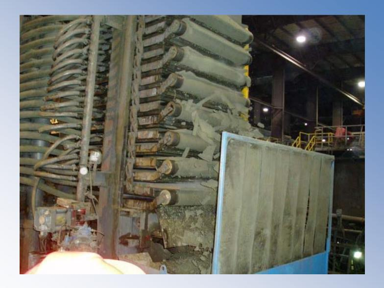
12. Multi-level filter press squeezes out water from the concentrate. From there the moist concentrate enters a gas-fired drier that heats the concentrate and lowers the water content to ~7%.
