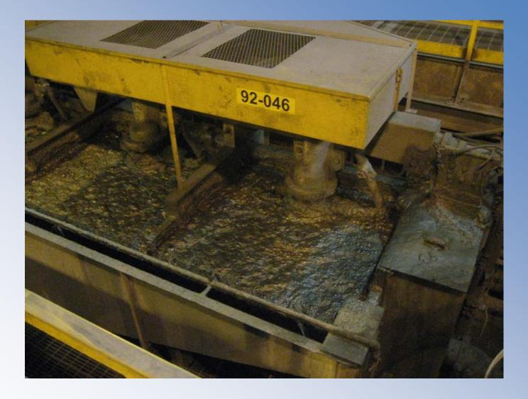
8. The reagent added causes the air bubbles rising through the slurry to collect or attract the fine ore particles, while the waste rock sand sinks to the bottom of the cell. (Tailings from the flotation cells are commonly directed by pipe to a nearby man-made tailings pond.)
