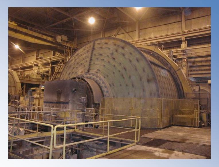
3. The ore is fed into one or a series of mills where it is mixed with water and tumbled continuously until the cobble size ore is reduced to the size of sand.
