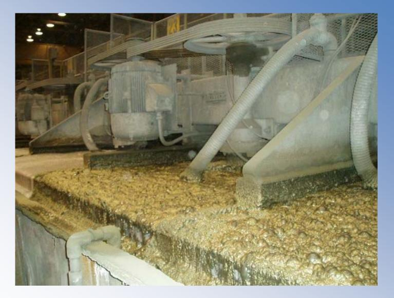
9. The frothy ore concentrate overflows the top of the cell and is collected and directed to other series of flotation cells that separate the different sulphide minerals that may be present in the deposit.
