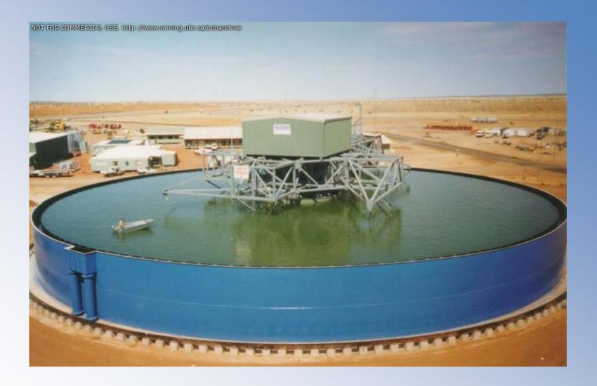
10. Collected frothy concentrates next enter thickening tanks where the concentrate settles and water content is reduced. At many operations this tank is enclosed in the mill.
