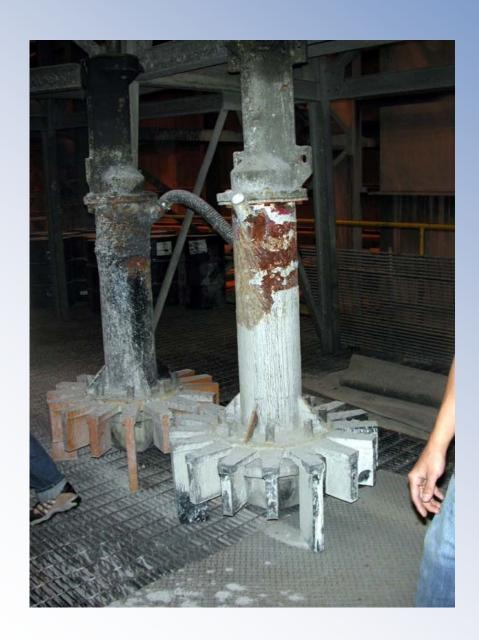
7. Aerator – steel device that sits in the middle of a flotation cell, agitates like a washing machine and feeds air into the slurry.
