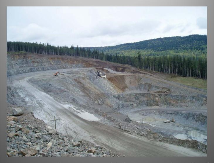
Open pit mining is used to extract ore in rock bodies that are at or close to the surface of the Earth. Large-scale equipment - drills, shovels, and trucks - are used to make operations efficient and economical. When they move in, the ore is dug up and sent to a mill for processing and reclamation procedures are initiated.
