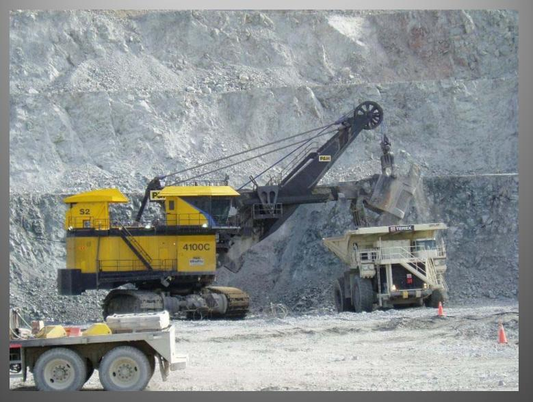
4 – Large electric or hydraulic shovels scoop up blasted rock and load into haul trucks.
