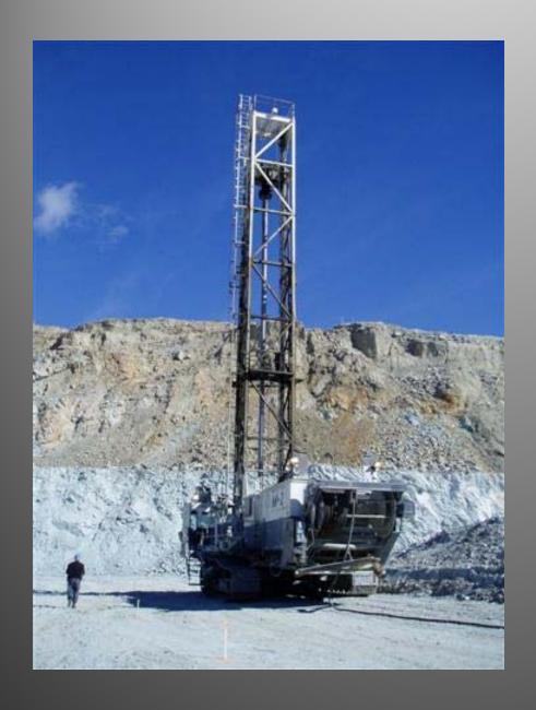
1 – In an open pit operation a rotary drill is used to drill holes that are ~30cm in diameter and ~15m deep. The holes are commonly filled with ANFO (short for ammonium nitrate fuel oil) explosives.
