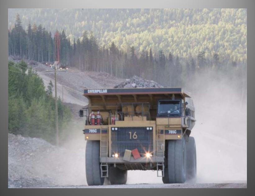
7 - Haul trucks also transport waste rock from a blast out of the pit to a waste rock dump.
