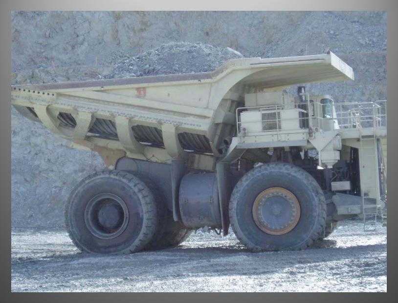
5 - Haul trucks loaded with ore transport it to a primary crusher which crushes the ore to pieces less than 30 cm.
