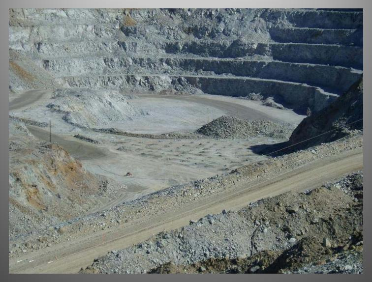
2 – The blast pattern – drill hole location and spacing and location - depends on the type of rock mined and overall mine plan. The depth of the hole will determine the height of the bench in the pit, generally 12-13m.
