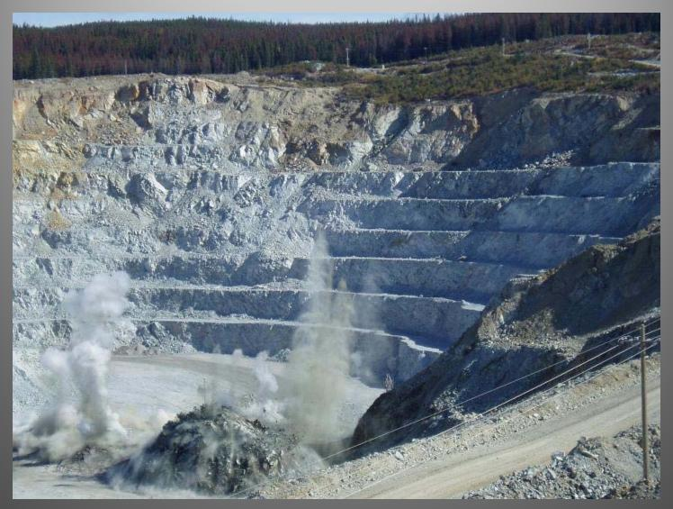
3 – Blasting! Explosives in the drill hole are detonated, breaking up the rock into smaller pieces that can be transported for further processing. Depending on the size of the mine, availability of equipment, and capacity of the mill, blasting may be scheduled every day or every 2-3 days.
